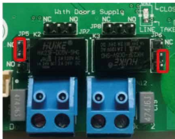
Relay 1: NC Relay 2: NO
